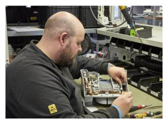
In the final assembly, mechatronic technician Christian Tilker unites the switch housing with its interior.
